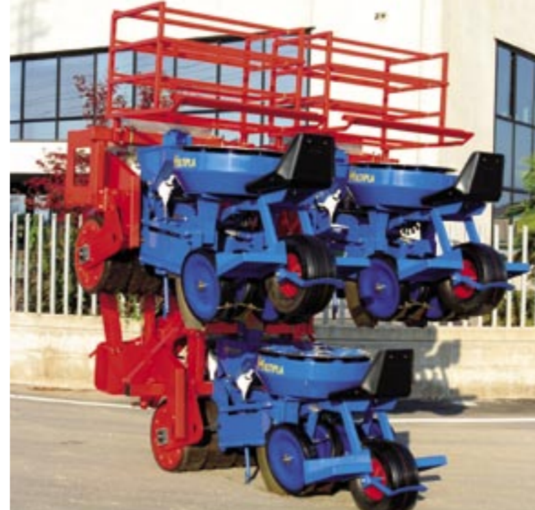
INGOMBRO MINIMO 2,5 m. / CLOSED HYDRAULIC BAR m. 2,50 BARRE HYDRAULIQUE FERMEE 2,50 metres FLEX-VORDERWALZE HYDRAULISCHER STAB - ZU = 2,50 meter / BARRA HIDRÁULICA CERRADA - m 2,50
